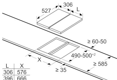
When installing two or more Domino units side-by-side, one or more assembly kits are required (2 units = 1 assembly kit, 3 units = 2 assembly kits, etc.).
